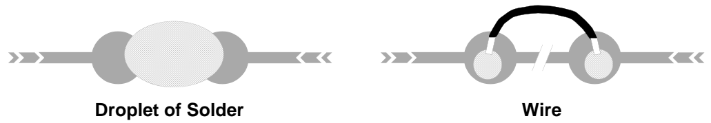
Figure 2. Configuration Pad - Re-connection
